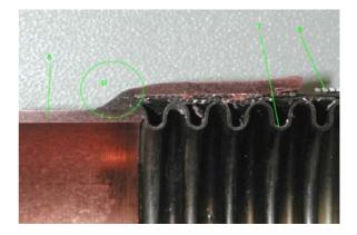
Part # 6 is the copper end, part # 7 is the flexible hose, part # 8 is the braiding and part # 9 is the ferrule.
