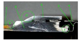
Part # 1 is the copper end, part # 2 is the transition ring in stainless steel, part # 3 is the flexible hose, part # 4 is the braiding and part # 5 is the ferrule. The first welding, marked A, unites the copper end to the transition ring; the second welding, marked B, unites the transition ring to the flexible hose; the third welding, marked C, unites the braid and the ferrule to the transition ring. All weldings are erformed in TIG or laser within argon protected environment.
