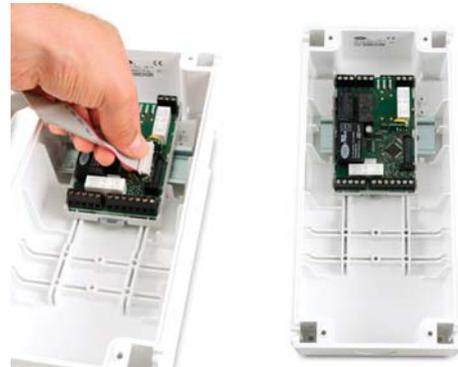
2. Release flat connector to remove frontal panel
