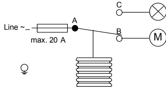
**Fig. 2: A - B open on pressure increase**
