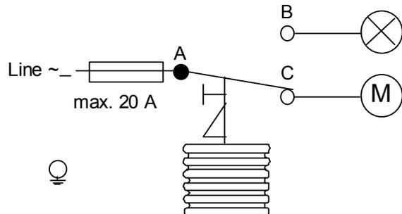
**Fig. 3: A - C open on pressure increase**
