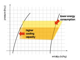
The extended operating range of the E<sup>X</sup>V means the refrigeration unit can work with floating condensing pressure, and consequently at the minimum allowed for the ambient temperature. This brings significant energy savings in all refer applications.
