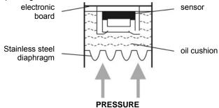
The protective stainless steel diaphragm ensures compatibility with the media frequently encountered in refrigeration systems. The outside of the PT4 consists of a corrosion resistant stainless steel enclosure. It is sealed at the electrical connector socket and at the pressure connector joint. This way, the PT4 meets the requirements of IP65.
