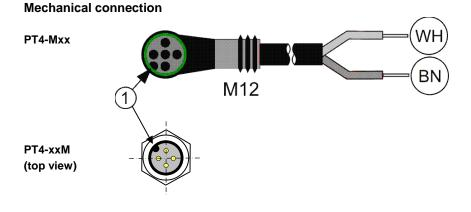
The PT4-Mxx cable assembly can only be fitted onto the PT4 Pressure Transmitter one way. Locate the corresponding lug shown as (1) opposite.
