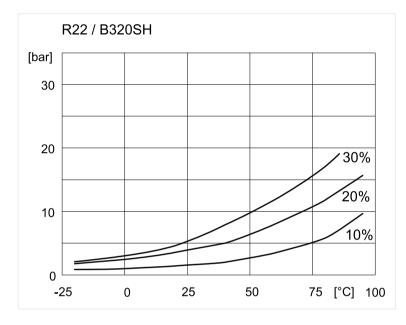
Oil B320SH: Refrigerant pressure depending on oil temperature and refrigerant content (mass % of refrigerant in oil-refrigerant blend).
