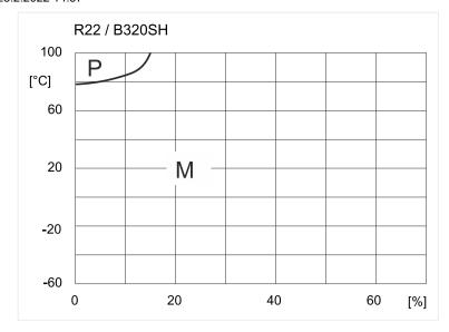
Miscibility gaps for oil B320SH: Limit temperature depending on oil content (mass % of oil in oil refrigerant blend).
