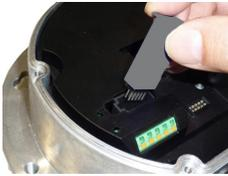
Example: Sticking the "FCC/IC" label onto a fan housing
