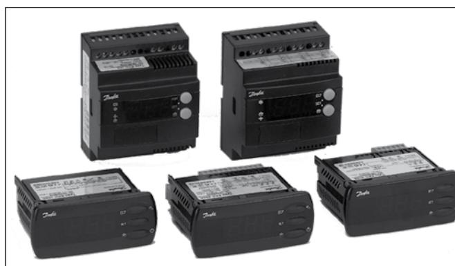
EKC 301 as DIN-rail mounting controller is designed for room temperature control via pump down or compressor start/stop. EKC 301 is controlling compressor, fan, defrost and alarm and it replaces several traditional controllers and defrost clocks due optional Real time clock module.
