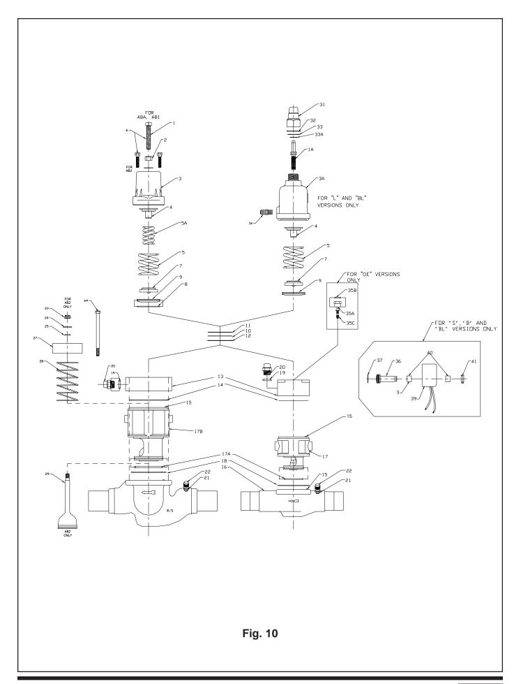
**THE SOLENOID FEATURES:** "S" for Shut-off, "B" for Bypass. To effect either of the features, a Solenoid is employed to modify the Pilot Stream at the Pilot Adapter. The Actuator is Normally Closed for both features, and can accept a variety of different coil voltages.
