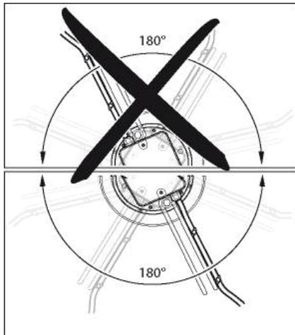
Fig. 3: Cable routing for fans installed upright.
