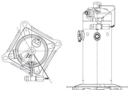
**Figure 2. DTC valve installation**
