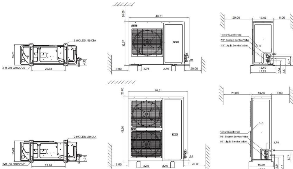
Figure 2 Unit dimensions and clearance Requirement
