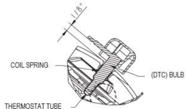
**Figure 6. Bulb installation on top of the compressor**
