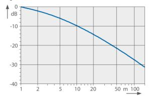
Fig. IV: Reduction of sound pressure level
