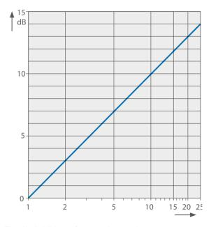
Fig. II: Addition of several sound sources
